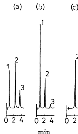
Fig. 4. Chromatograms of a mixture of Ni(DEDTC) 2 , Ni(PAN) 2 , and Ni(DMG) 2 . Column: Shodex silipak (4 mm × 15 cm). Eluent: hexane:ethyl acetate=100:25 (water saturated). Flow rate: 3.2 cm 3 /min. Detector: (a) 254 nm, (b) 325 nm, (c) 530 nm. Sample sizes: 5 μl. 1: Ni(DEDTC) 2 , 2: Ni(PAN) 2 , 3: Ni(DMG) 2 .
