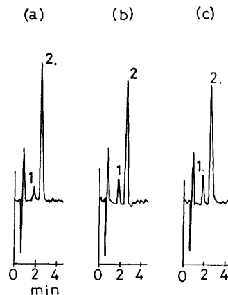
Fig. 2 Change of chromatogram patterns by ligand exchange. Column: Shodex silipak (4 mm \times 15 cm). Eluent: hexane : ethyl acetate = 100 : 8 (water saturated). Flow rate: 2.5 cm 3 /min. Detector: 325 nm. Sample size: 200 \mu l (in chloroform: ethyl acetate: hexane = 1 : 1 : 8). Sample: 5.0 \times 10^{-6} mol dm -3 Ni[(C_2H_5)_2NCSS]_2 ( =MA_2 ) + 7.9 \times 10^{-7} mmol dm -3 (C_3H_7)_2NCSS^- ( =B ). (a) After mixing 15 s, (b) 35 s, (c) 3 min (equilibrium). 1: NiAB, 2: NiA_2 .
